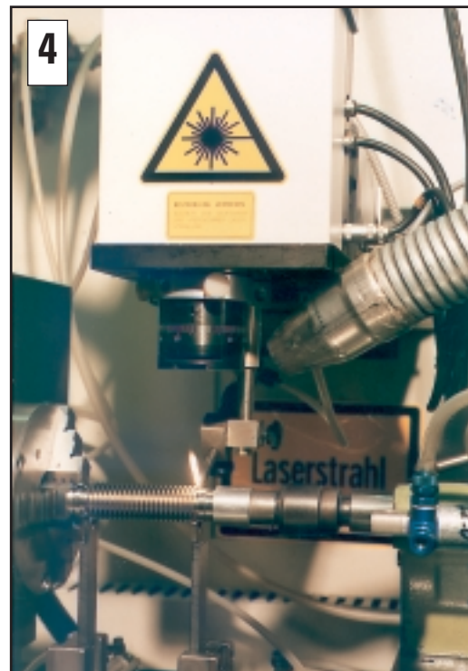
4 Laser welding of bellows to end rings.
