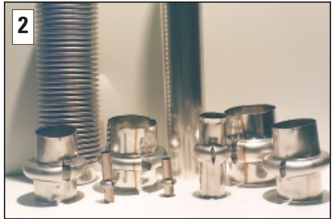
2 In-line inspection of tube welding prior to convolution forming.
