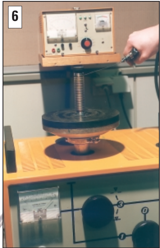
6 Helium leak testing. Bellows are rejected if leakage exceeds 10^{-8} cm 3 per second.
