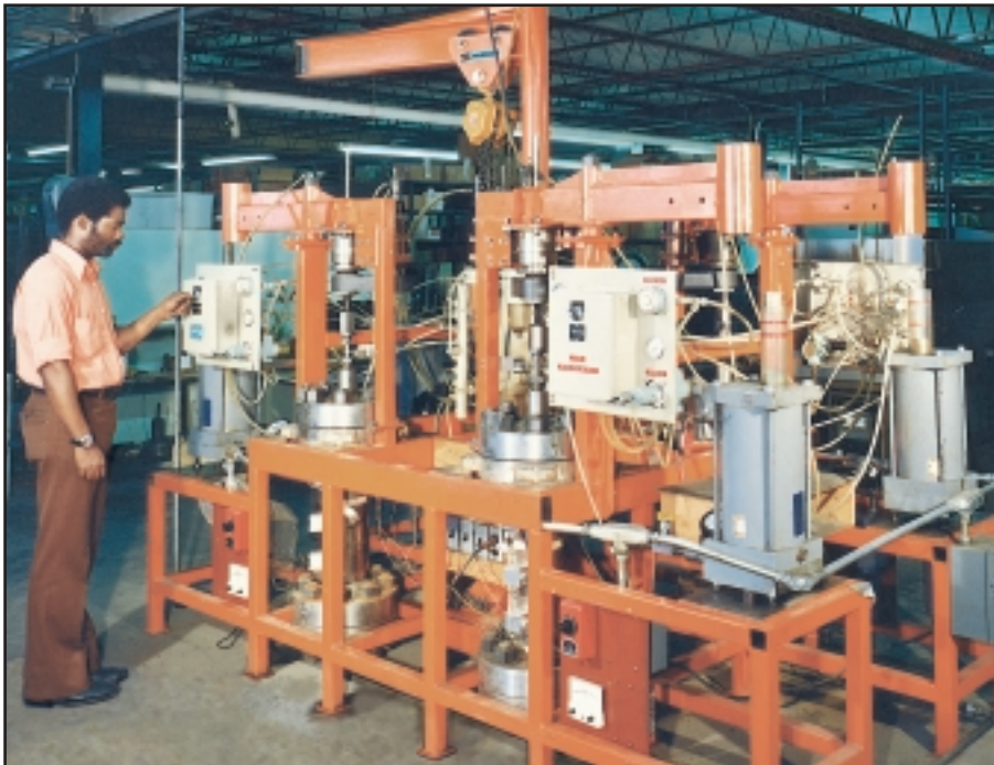
Hot loop for cycling four bellows seal valves at 1800 psig @ 650°F (124 bar @ 343°C).
