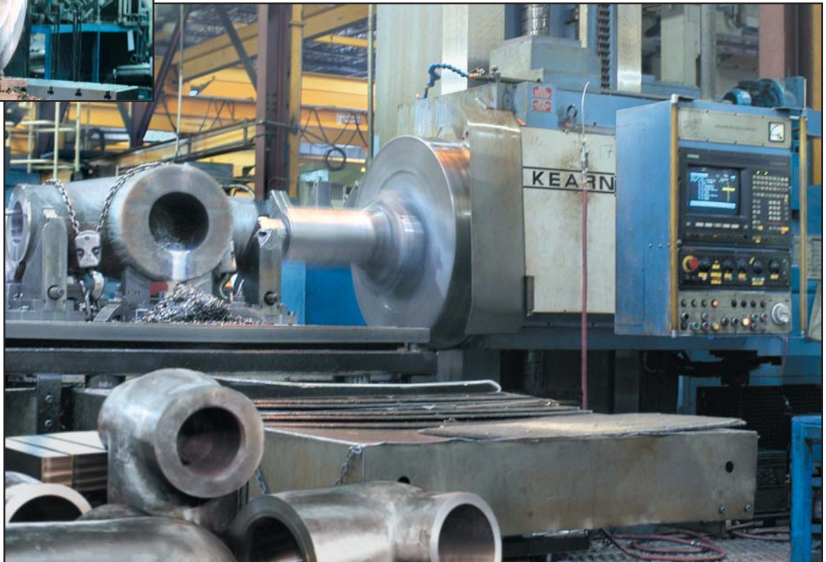
A large CNC horizontal boring mill (with tool changers) machining forged pressure seal bodies.
